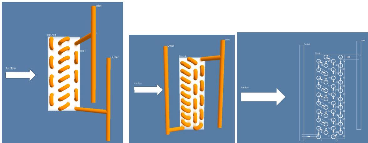
**Figure 6: Original design (left: 32 tubes, 9.52 mm, single path) and prototype design (middle and right: 40 tubes, 5 mm, single path) for R290 condensers.**
