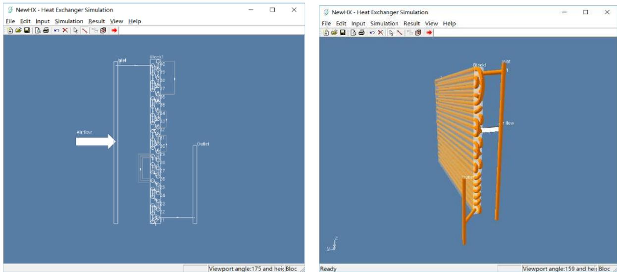
**Figure 2: Tube circuitry is specified by linking tube ends together in a two-dimensional graphical interface. A three-dimensional visualization of the circuitry is then produced.**
