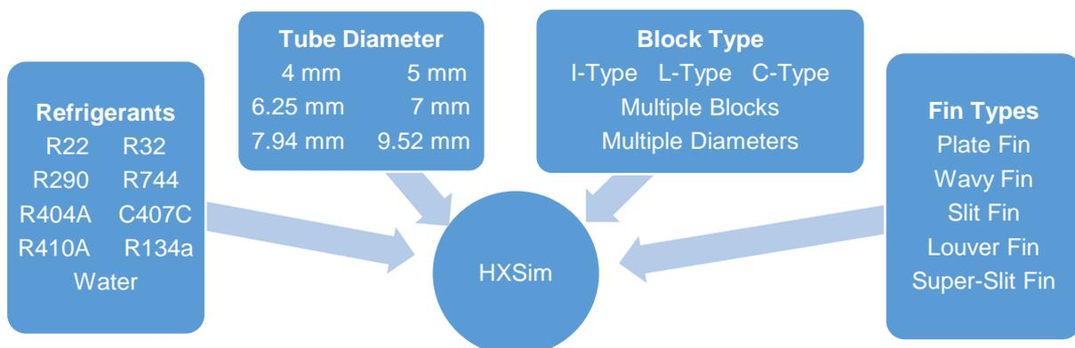
**Figure 1: Tube diameter, block type, refrigerants, fin types and other parameters are input via menu choices within the HXSim software program.**
