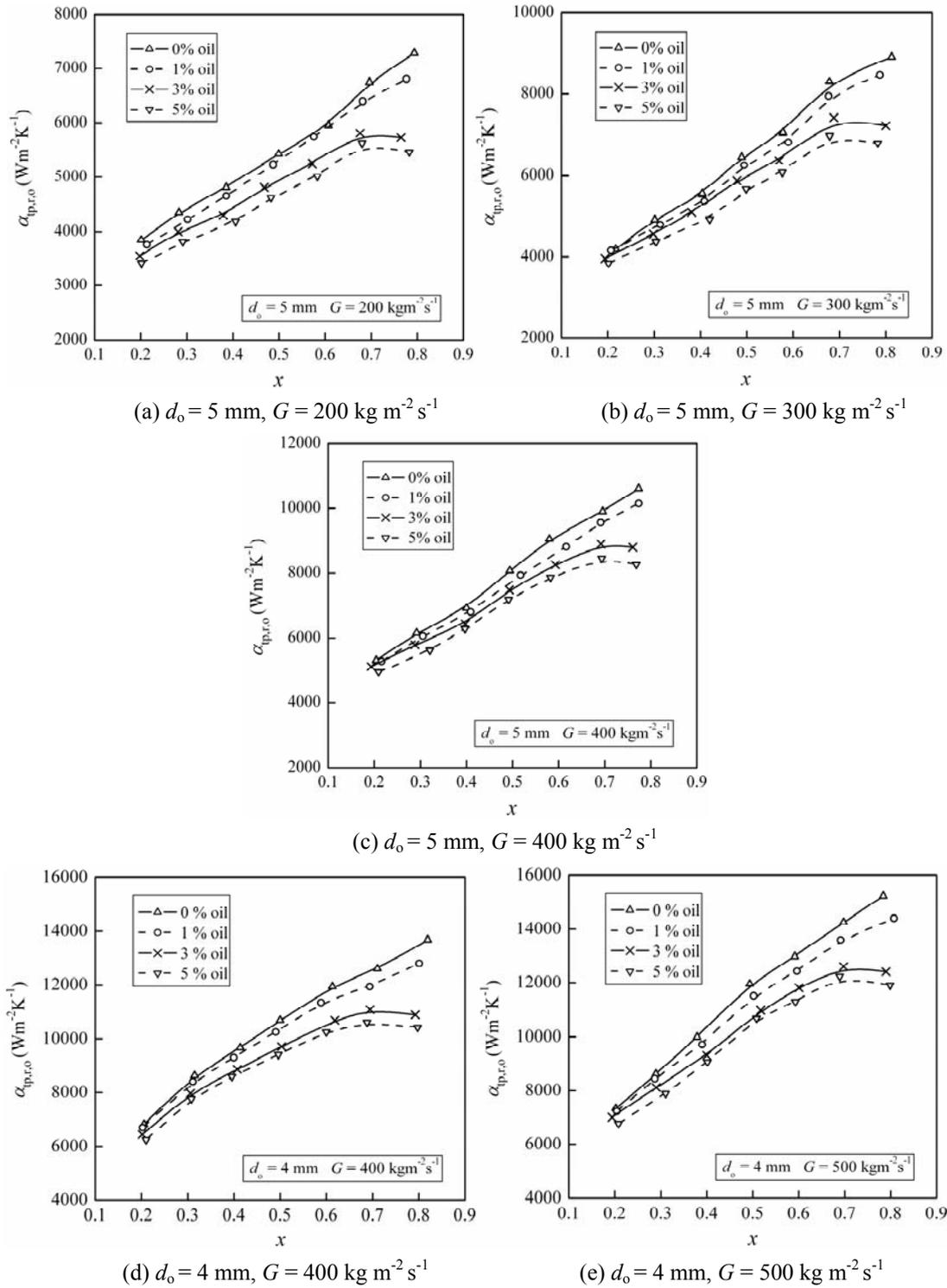
**Fig. 3. Heat transfer coefficients of R410A-oil mixture flow condensation inside 5 mm and 4 mm O.D. microfin tubes as a function of vapor quality at different mass fluxes**
