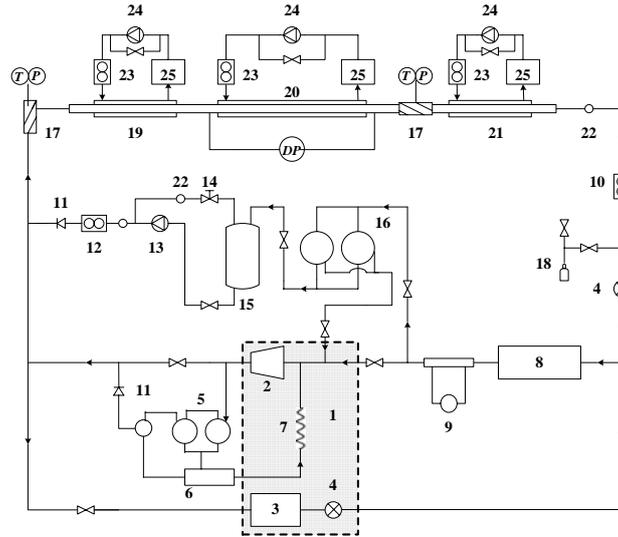
1-Outdoor unit, 2-Compressor, 3-Condenser, 4-Electronic expansion valve, 5-Oil separator for compressor, 6-Oil container, 7-Capillary, 8-Indoor unit, 9-After-heater, 10-Refrigerant mass flowmeter, 11-Check valve, 12-Oil mass flowmeter, 13-Oil pump, 14-Regulating valve, 15-Oil tank, 16-Oil separator for test section, 17-Mixing chamber, 18-Sampling cylinder, 19-Pre-condenser, 20-Test section, 21-After-condenser, 22-Sight glass, 23-Water volume flowmeter, 24-Water pump, 25-Thermostat
