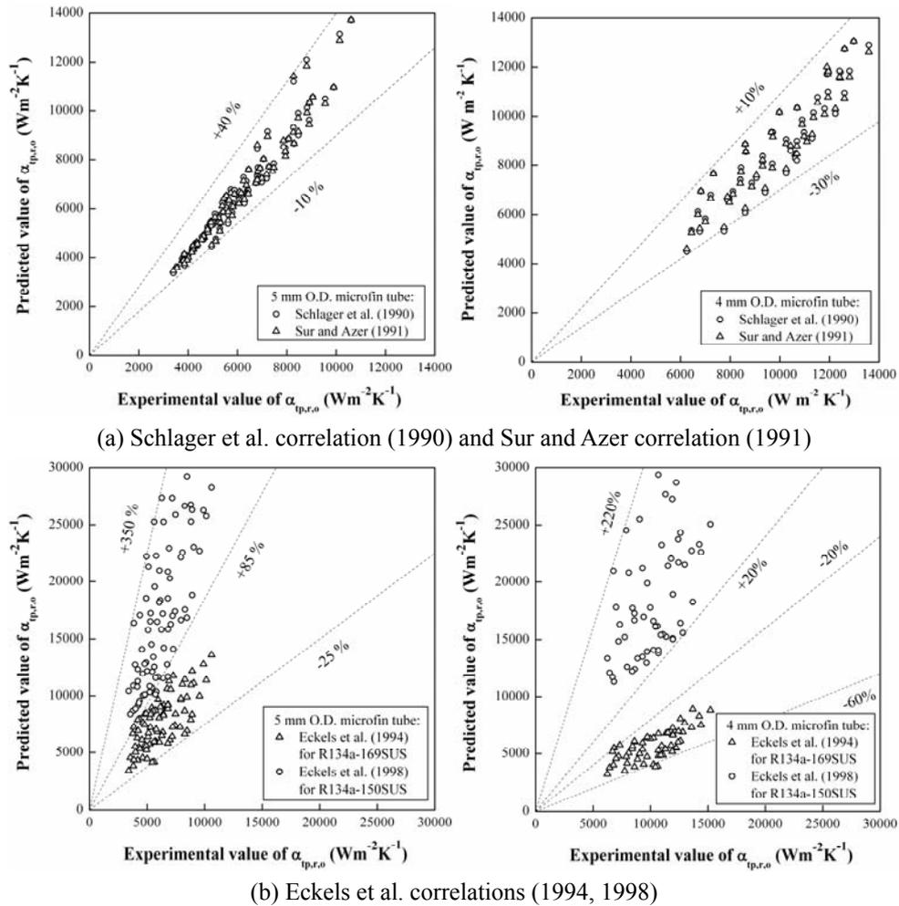
**Fig. 5. Comparison of experimental condensation heat transfer coefficients of R410A-oil mixture with the predicted values of EF correlations**
