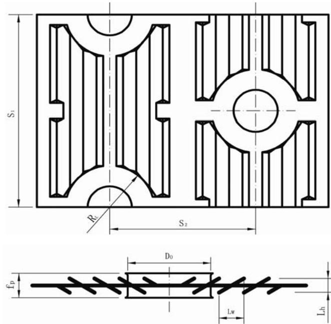
Fig.3 Schematic diagram of louvered fin
