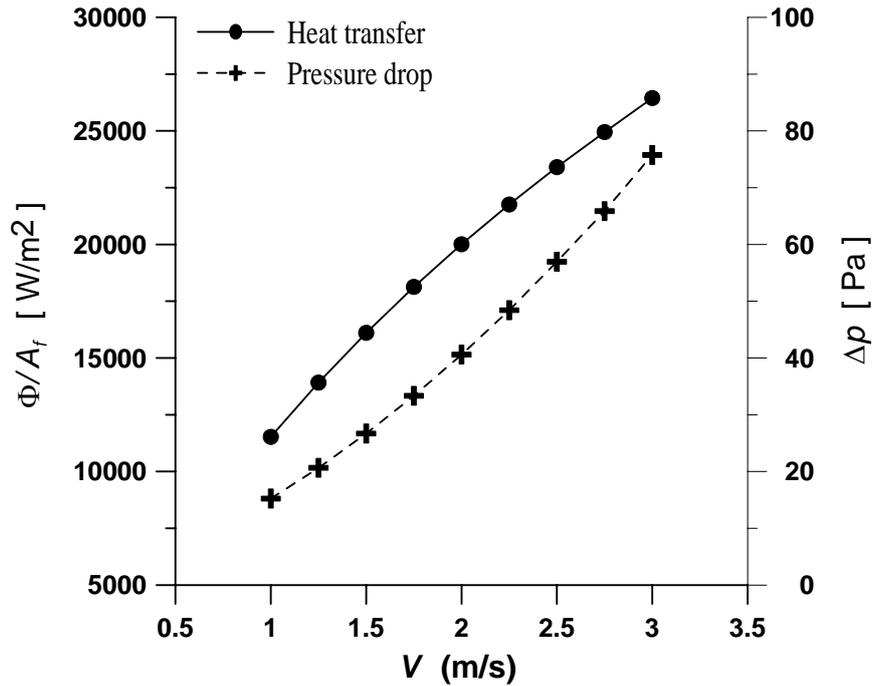
Fig.5 Heat transfer and pressure drop of reference fin
