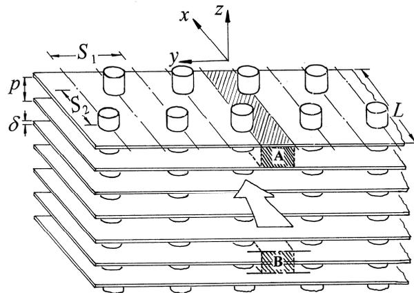
Fig.1 Pictorial view of plain fin-and-tube heat exchanger
