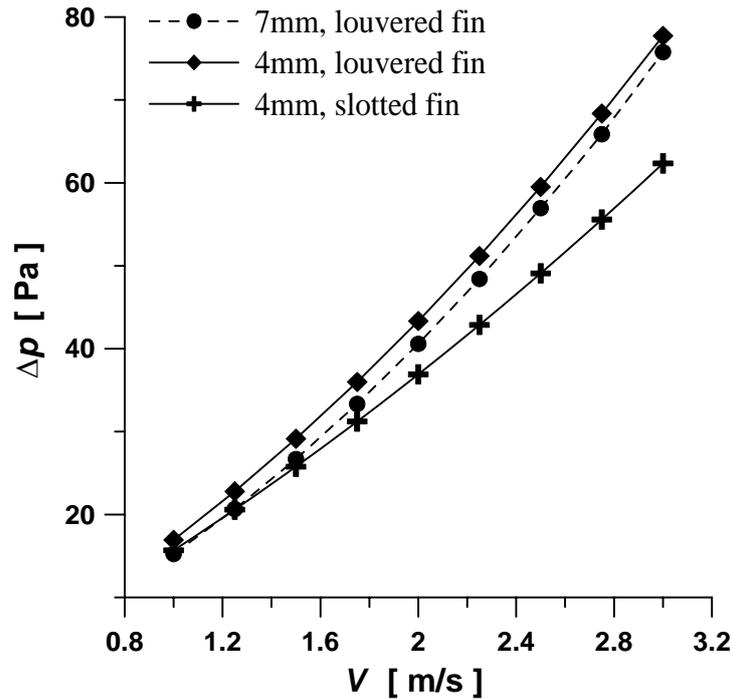
Fig.9 Comparison of pressure drop
