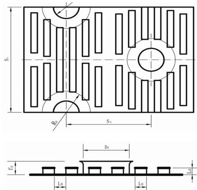
Fig.4 Schematic diagram of slotted fin
