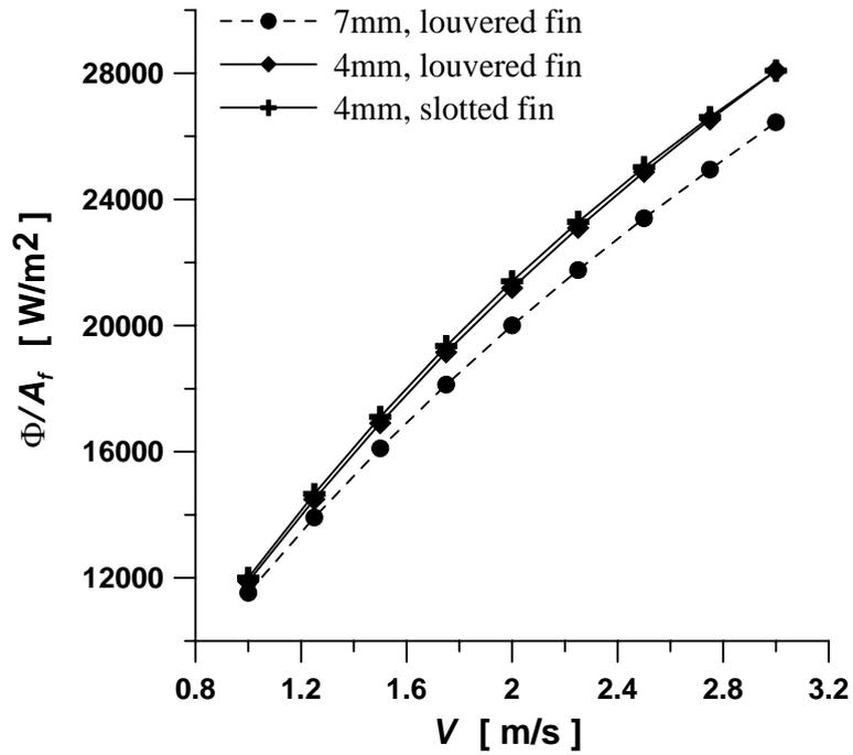
Fig.8 Comparison of heat transfer performance
