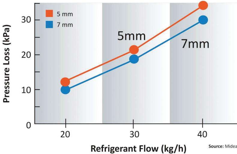
Figure 3. A smaller diameter tube results in a higher pressure drop for a given flow rate of refrigerant through the tube.
