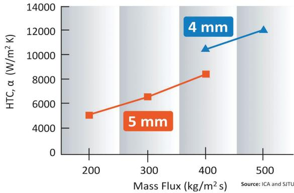
Figure 1. The local heat transfer coefficient increases as tube diameter decreases, which means more heat can be transferred using less coil material if the smaller tube diameters are used in coil designs.
