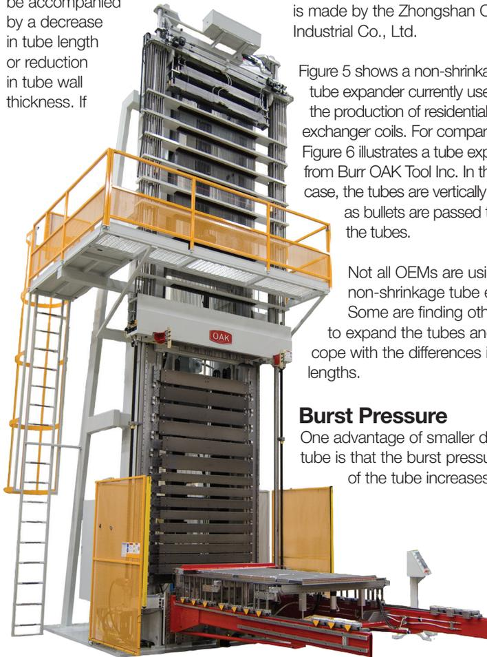
Figure 6. This vertically oriented tube expander made by Burr OAK Tool Inc. was specially designed for the expansion of 5-mm diameter tubes.
