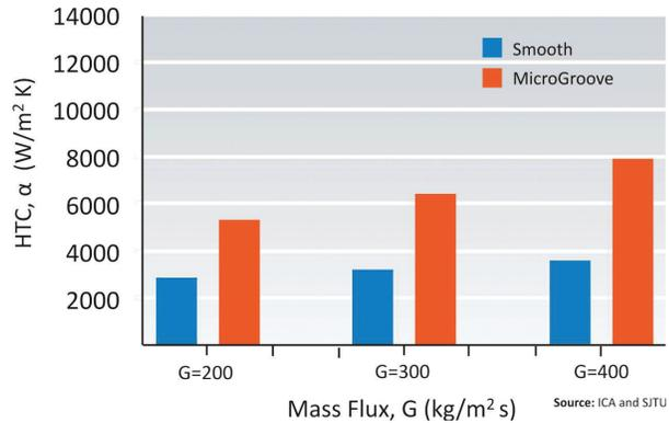
Figure 2. Inner grooves or “microfin” patterns can further improve the local heat transfer coefficients. (Data is from laboratory measurements on 5-mm diameter copper tubes with and without inside-the-tube surface enhancement.)
