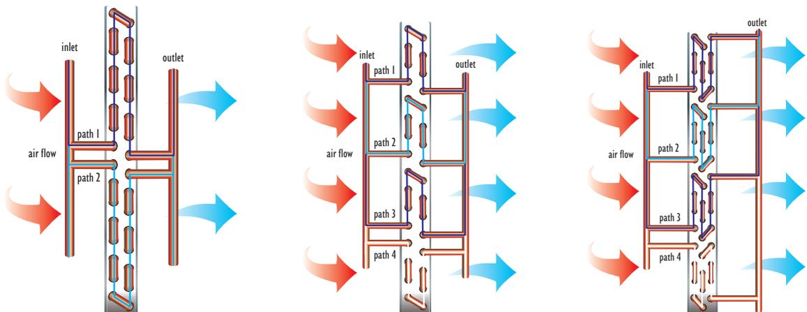
Figure 4. Tube circuitry can be adjusted to accommodate smaller diameter tubes.
