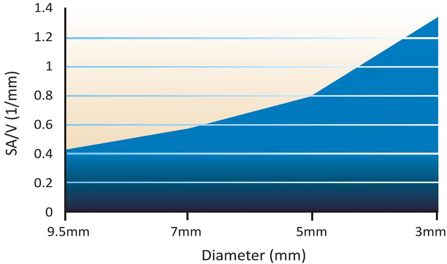
A plot of the internal surface area of a tube over internal volume shows that as tube diameter is reduced, the amount of surface area that is available in the same volume increases dramatically. With reduced tube diameters, more surface area is available to transfer heat.
