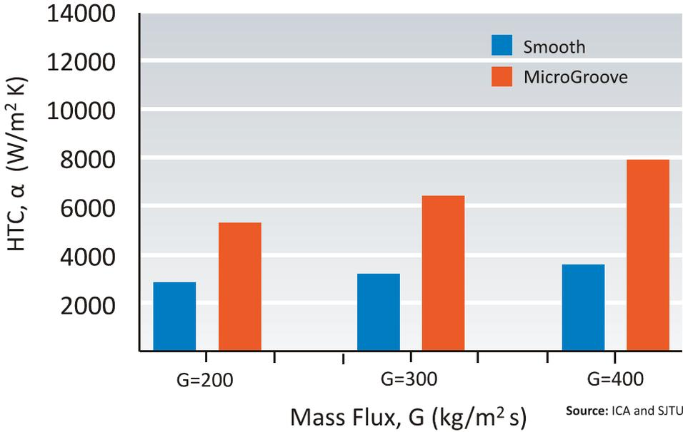
The effect of grooves and internal tube enhancements on the heat transfer coefficient can be seen above, measured in 5 mm tubes at three different mass flux rates using R410A refrigerant. The effect on the heat transfer coefficient when compared to a smooth internal tube surface is rather significant, as seen in this data.
