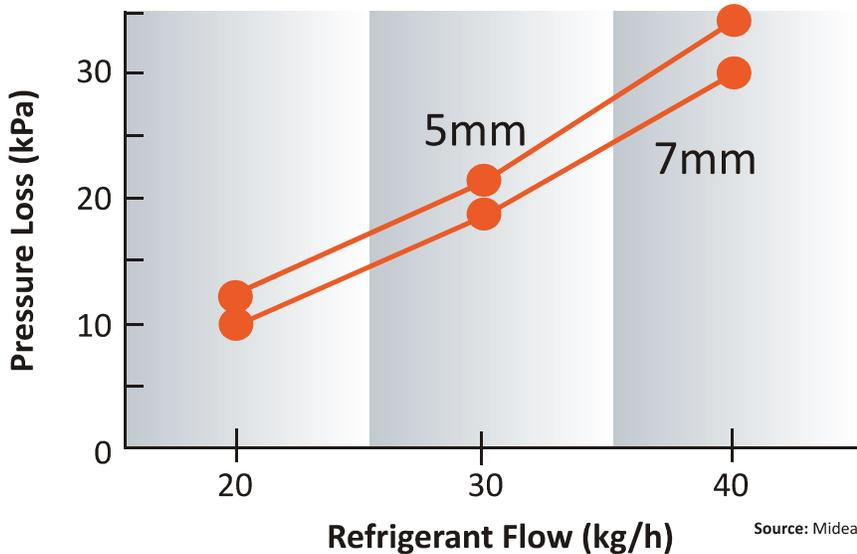
Pressure loss is plotted above, measured in an evaporator core with 7 mm tubes and one with 5 mm tubes. The refrigerant in this experiment was R410A. At three different flow rates, a slightly higher pressure loss can be seen in the smaller diameter tube. Pressure losses can be easily reduced with increased number of branches and reduced tube length per branch.
