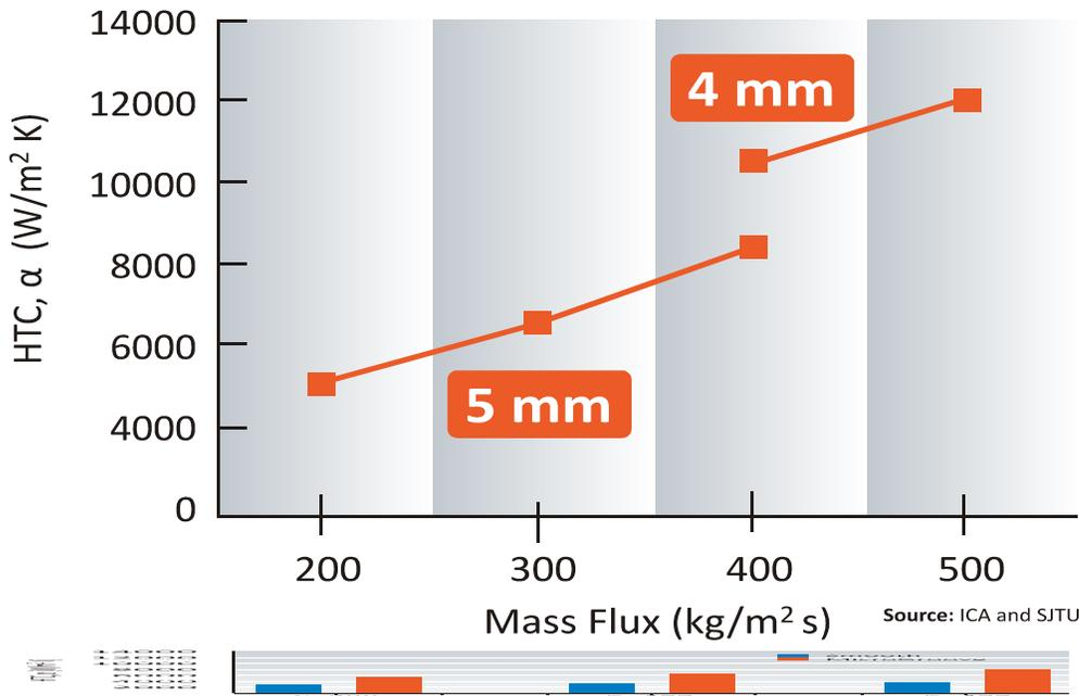
Above, the heat transfer coefficient is measured for 5 mm and for 4 mm MicroGroove tubes in a condenser using R410A as a refrigerant. Note that mass flux is defined as mass per area per time. Only the tubes were modified in this experiment leaving fins and external conditions constant. The higher heat transfer coefficient can be seen in the 4 mm tube. This phenomenon of increased heat transfer coefficient in smaller diameter tubes can be replicated with other refrigerants.
