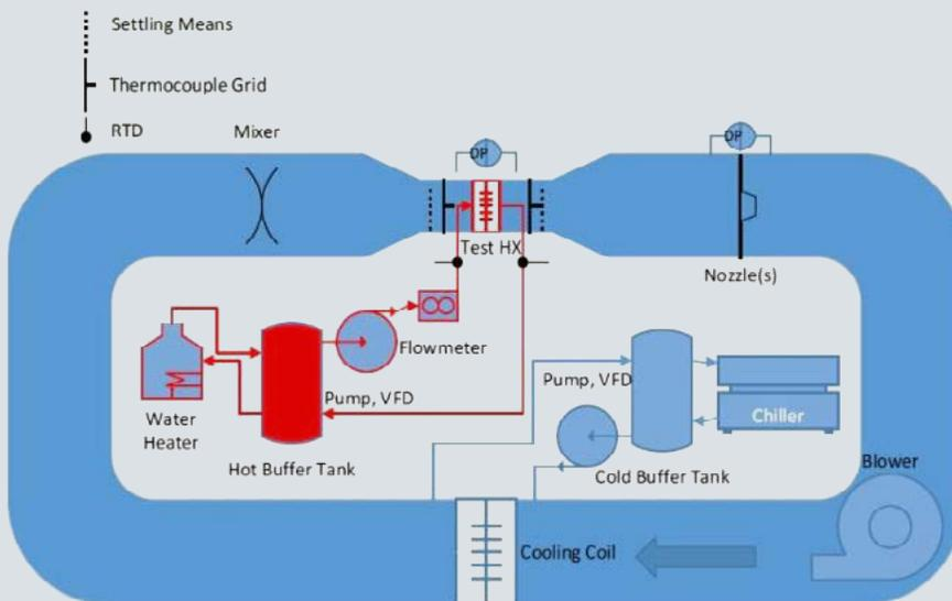
Here is a schematic of the heat exchanger test facility that was used to experimentally validate the MicroGroove correlations that are used in CoilDesigner software. Dennis Natasa from OTS presented a [paper on this topic](#) at the 2018 Purdue Conferences.
