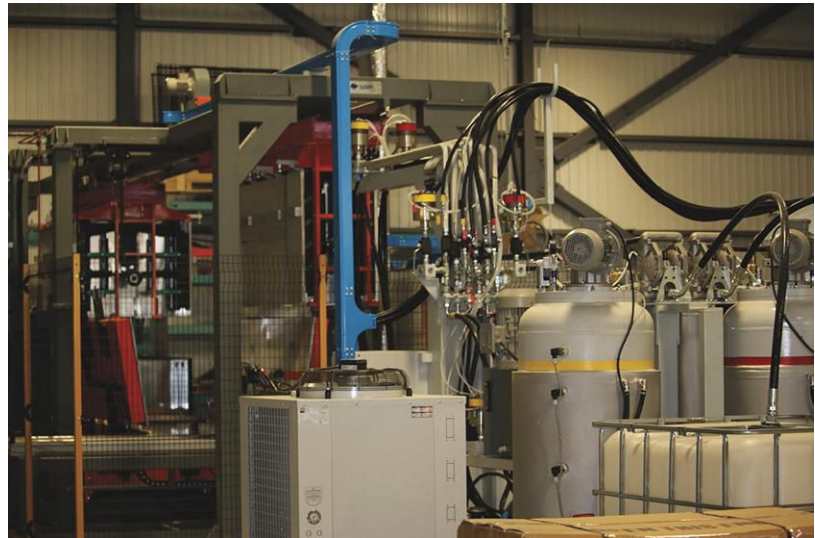
High-pressure polyurethane foam injection system, showing the two tanks for two foam components. (Courtesy of MTL Technologies)
