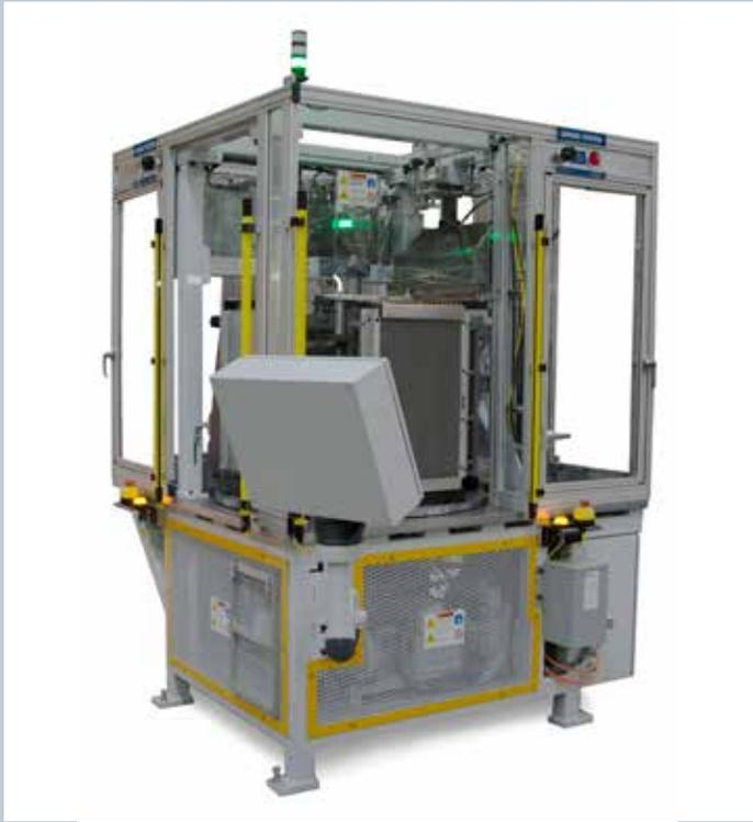
New equipment from OAK uses pressure to expand smaller-diameter copper tubes into fin plates. (Photography Courtesy of Burr OAK Tool Inc.)
