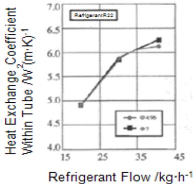
Figure 1 Heat Transfer Coefficient Comparison Within Tube
