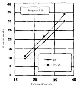
Figure 2 Comparison of Pressure Loss Within Two Kinds of Copper Tubes
