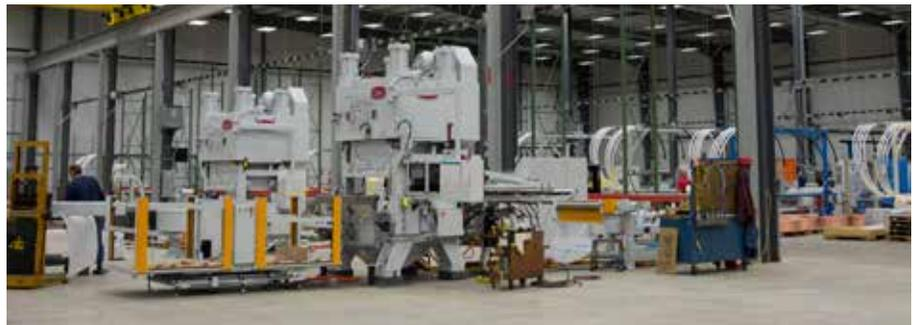
New equipment in the fin line includes presses for fin stamping. (Photograph courtesy of BOTI.)
