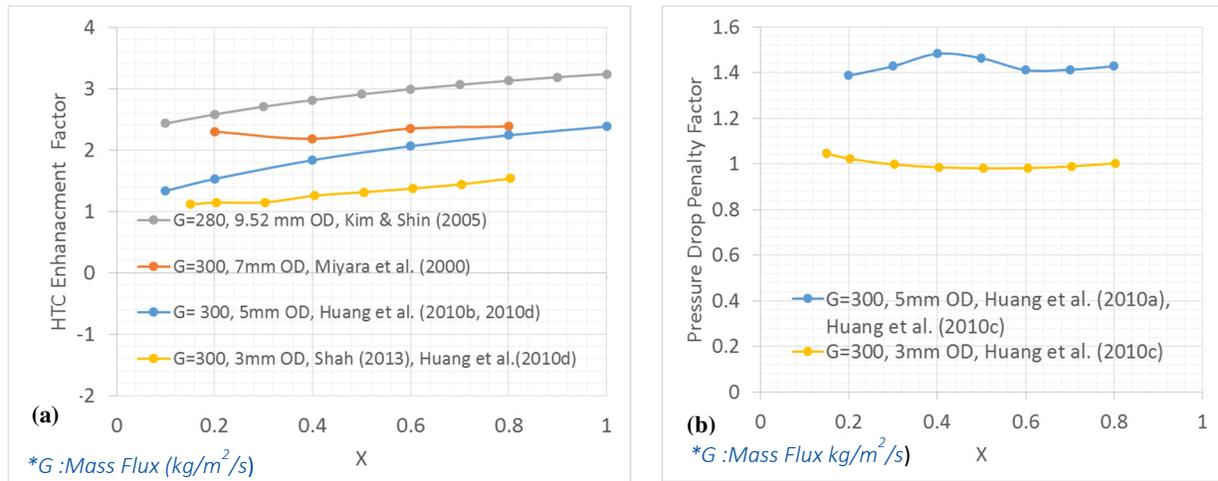
**Figure 5. Influence of vapor quality and tube diameter on (a) HTC Enhancement Factor and (b) Pressure Drop Penalty Factor for helical microfinned tube.**
