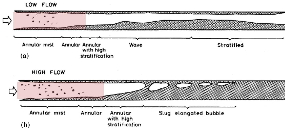
**Figure 2. Condensation flow pattern for (a) Low mass flux (Thome (2003)); and (b) High mass flux (Collier and Thome (1998))**
