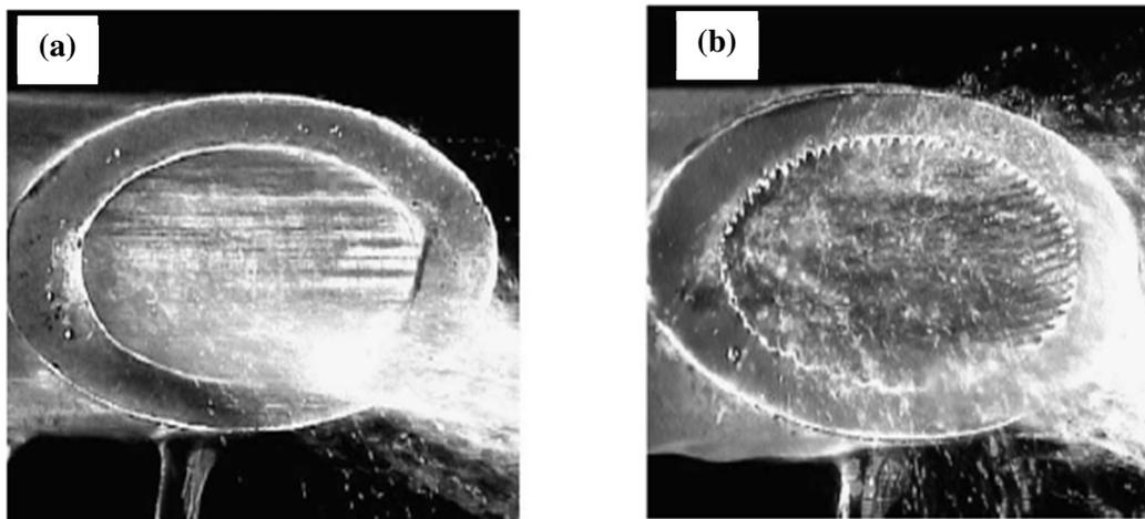
Figure 4. Influence of helical microfins on the flow pattern for (a) Smooth Tube – Stratified Flow Pattern; and (b) Microfinned Tube – Annular Flow Pattern (R134a,  $G=200 \text{ kg/m}^2/\text{s}$ ,  $x=0.5$ ,  $T_s=40^\circ\text{C}$ , OD=8 mm, Cavallini et al. (2003))
