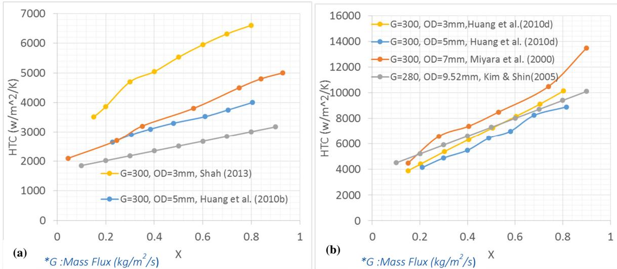
**Figure 6. Influence of tube diameter on the HTC for (a) smooth tube ; (b) microfinned tubes.**
