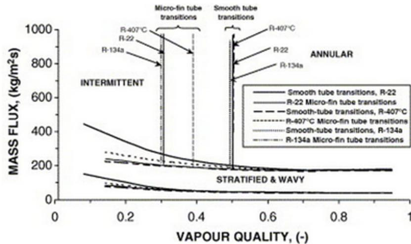
Figure 3. Flow pattern map for smooth and enhanced tube (Tube OD  $\approx$  9.5 mm) indicating how internal enhancement delays the transition of the flow from annular to intermittent, i.e., wavy and slug (Liebenberg and Meyer (2006))
