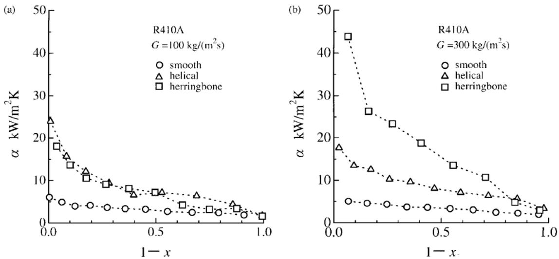
**Figure 7. Comparison of HTC for smooth tubes, helical microfinned tubes, and herringbone microfinned tubes for (a) small mass flux; and (b) large mass flux (All tubes had an OD = 7 mm, microfin height and width for both herringbone and helical-groove tube was almost identical. Miyara et al. (2000))**
