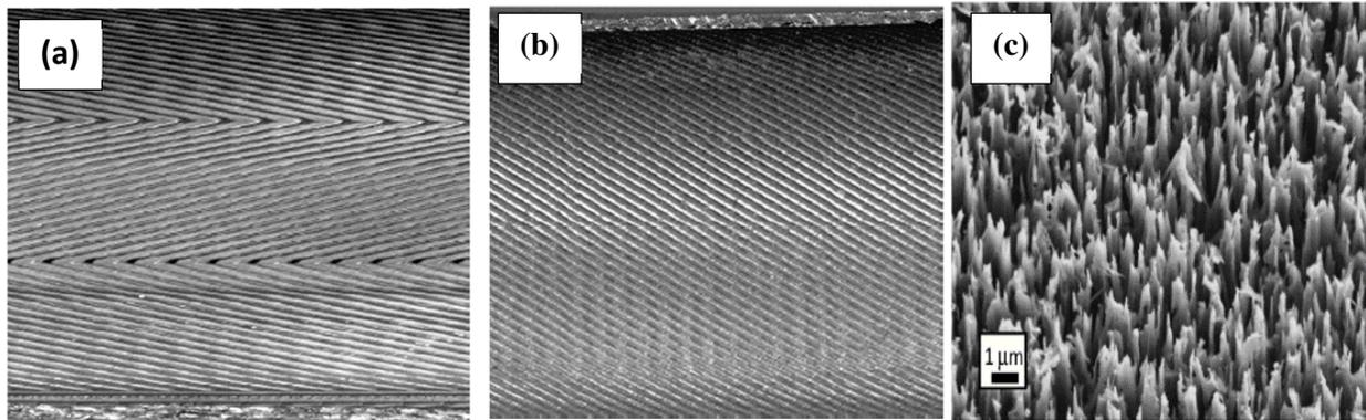
**Figure 1. Internal enhancements to augment the heat transfer on refrigerant side. (a) Herringbone fins; (b) helical microfins; (c) microstructures.**
