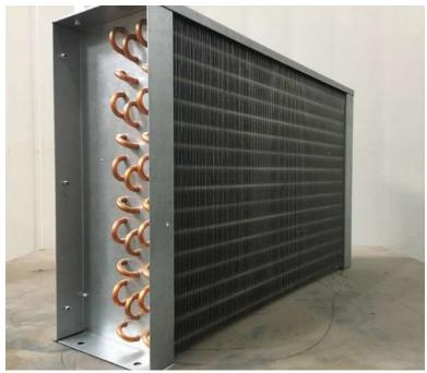
Photographs of C1 Prototype with sixty 5 mm copper tubes of 420 mm length in four rows.
