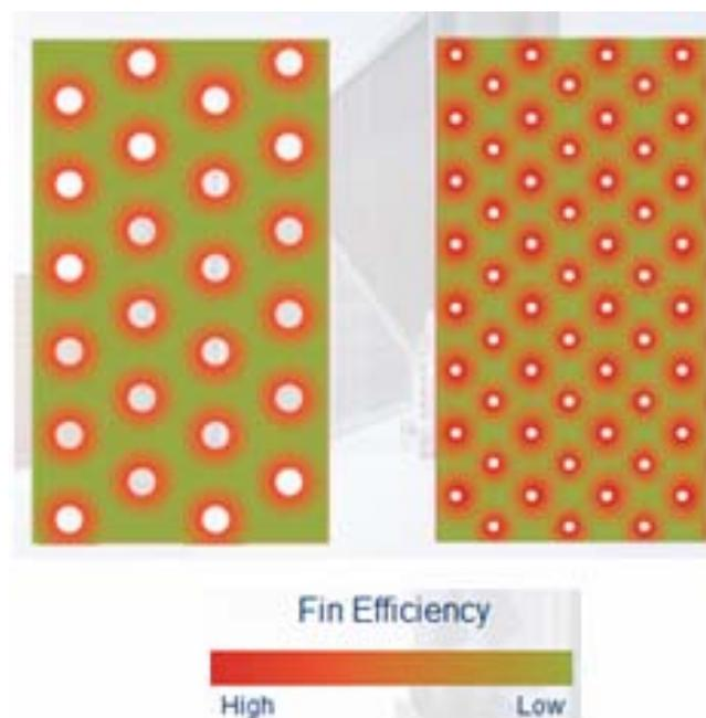
Figure 5. Fin hole patterns for 9.52 mm tube (left) and 5mm tube (right) show more primary heat transfer effective area for the smaller diameter tubes.
