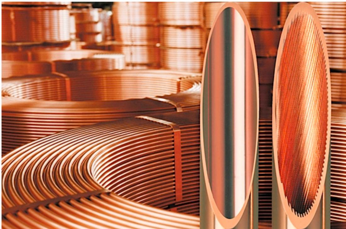
Figure 2. Smooth or inner-grooved tubes made of a high-strength copper alloy (CuFe2P) are suitable for high pressure applications using R744. The CuFe2P alloy consists of copper alloyed with Fe (2.1 to 2.6 wt. %), Zn (0.05 to 0.20 wt. %), P (0.015 to 0.15 wt. %) and Mg (0.10 max. wt. %). Wall diameters range from 0.25 mm to 2.0 mm.
