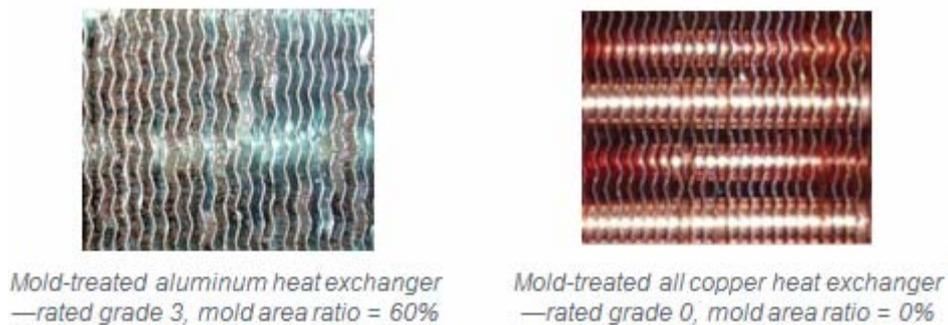
Figure 4. A mold-treated heat exchangers made of copper were unaffected by mold growth while the heat flow rate of a mold-treated aluminum heat exchanger dropped by 19 percent (Ding, 2007).
