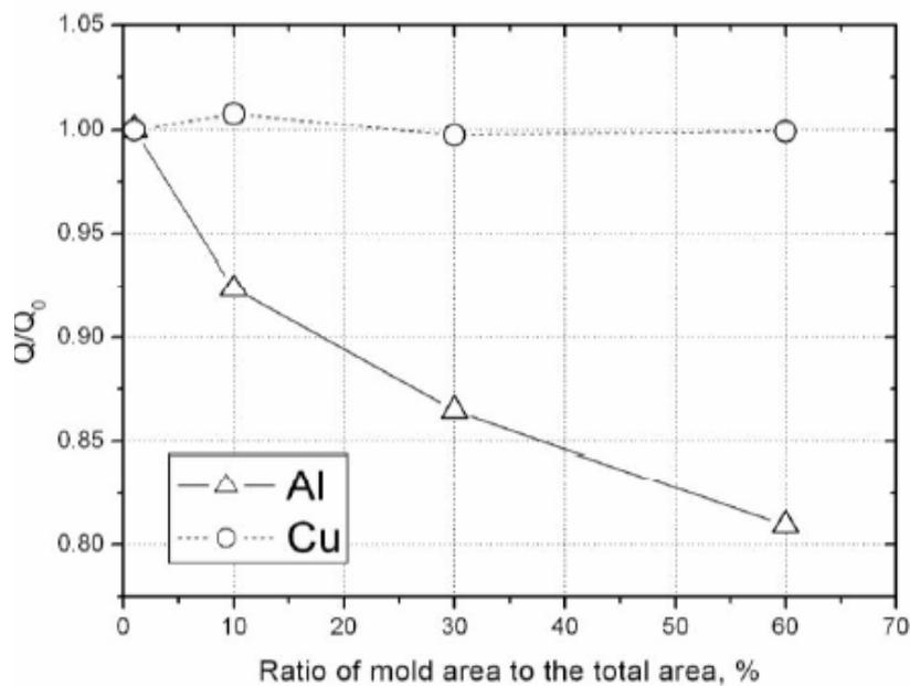
Figure 5. Normalized heat flow to mold growth area on aluminum fins and all-copper heat exchangers with mold areas of 0, 10, 30 and 60 percent. Performance declined 19 percent with aluminum fins while it remained unchanged with copper fins (Ding, 2007).
