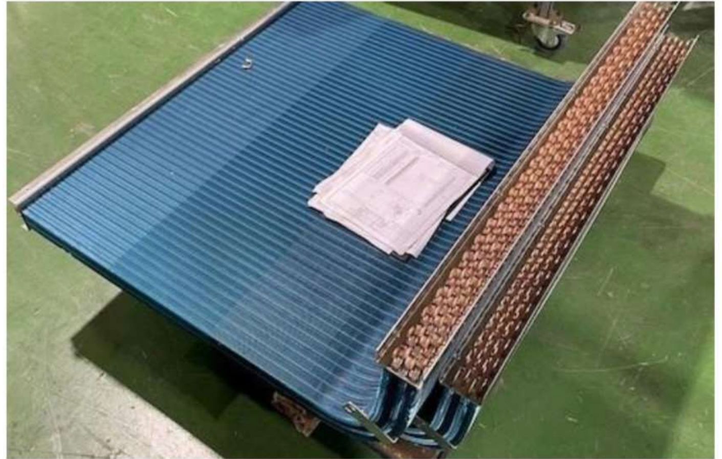
Photograph of the actual evaporator on factory floor prior to brazing of the inlet and outlet distributor lines
