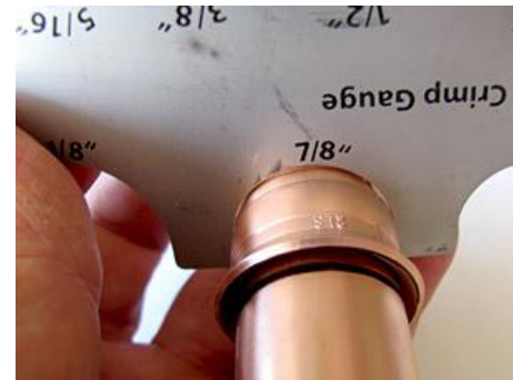
Properly crimped joint
