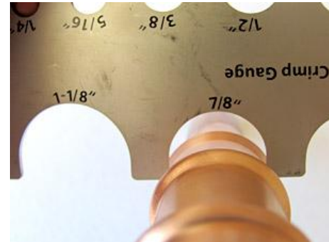
Improperly crimped joint
