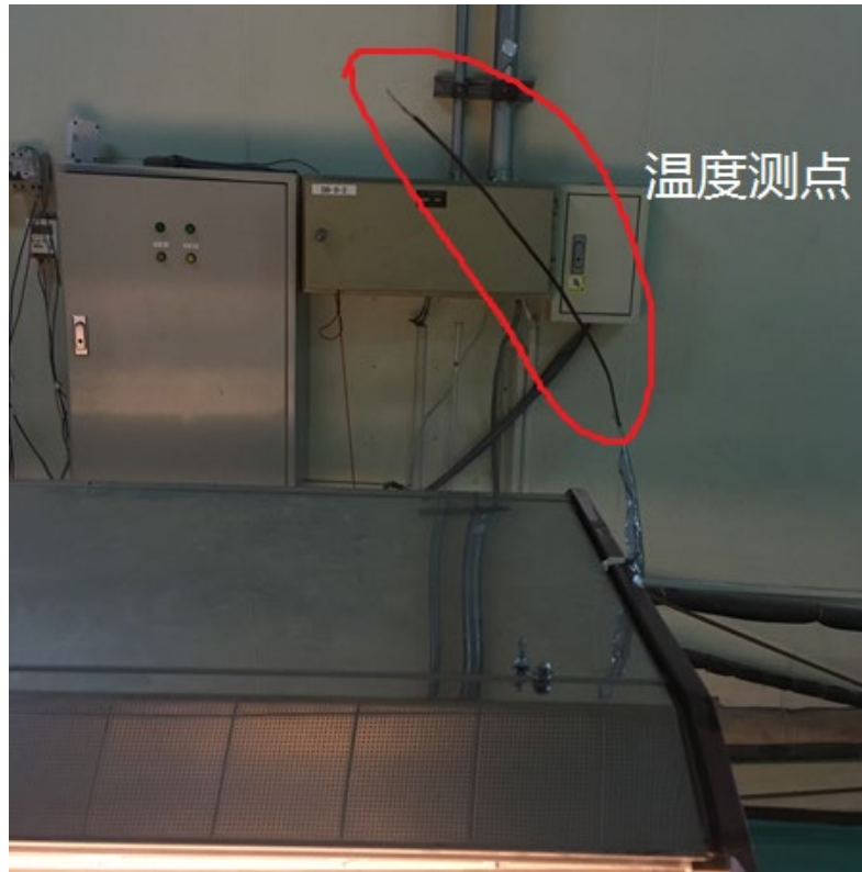
Figure 1-3 Layout of ambient temperature measurement points
