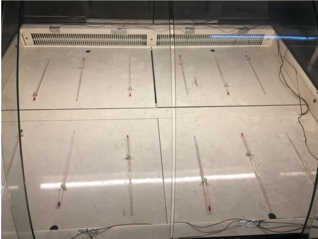
Figure 1-10 Display surface thermometer arrangement
