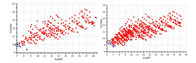
Figure 8. Optimization (with respect to air side pressure drop) study for 5 mm (a) smooth tube; (b) microfined tube.
