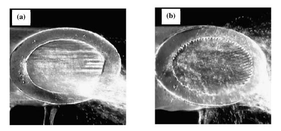
Figure 4. Influence of helical microfins on the flow pattern for (a) Smooth Tube – Stratified Flow Pattern; and (b) Microfinned Tube – Annular Flow Pattern (R134a, G=200 kg/m<sup>2</sup>/s, x=0.5,  $T_s$ =40°C, OD=8 mm, Cavallini et al. (2003))
