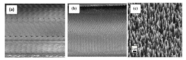
Figure 1. Internal enhancements to augment the heat transfer on refrigerant side. (a) Herringbone fins; (b) helical microfins; (c) microstructures.
