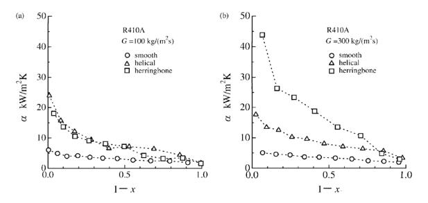
Figure 7. Comaprison of HTC for smooth tubes, helical microfinned tubes, and herringbone microfinned tubes for (a) small mass flux; and (b) large mass flux (All tubes had an OD =7 mm, microfin height and and width for both herringbone and helical-grove tube was almost identical. Miyara et al. (2000))
