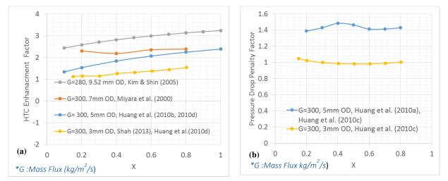
Figure 5. Influnce of vapor quality and tube diameter on (a) HTC Enhahncement Factor and (b) Pressure Drop Penalty Factor for helical microfinned tube.
