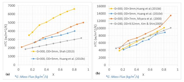
Figure 6. Influence if tube diameter on the HTC for (a) smooth tube ; (b) microfinned tubes.
