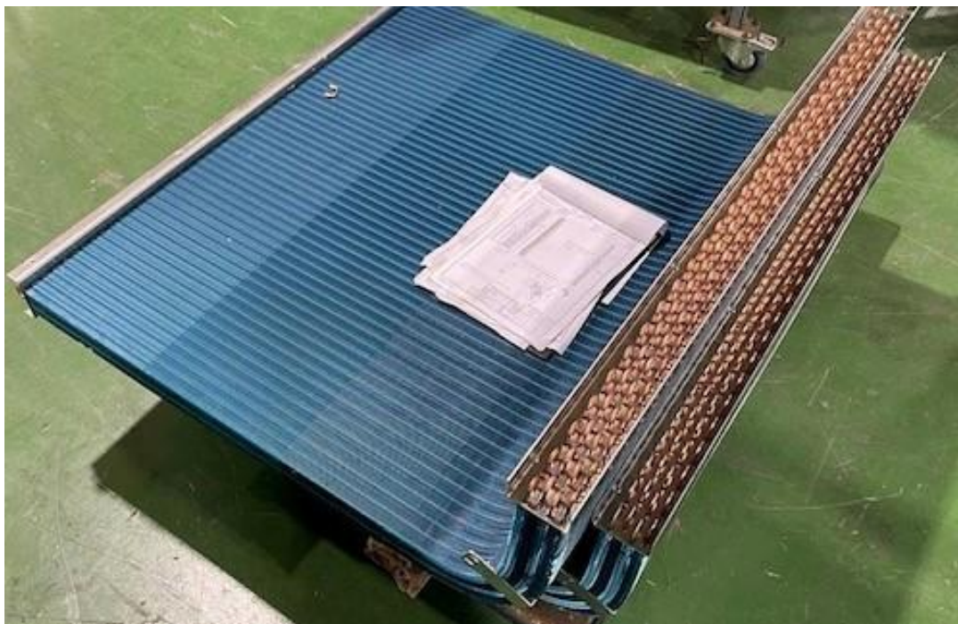
Figure 3: Three-dimensional simulation results with temperature map for 15 kW evaporator (top) and photograph of the actual evaporator on factory floor prior to brazing of the inlet and outlet distributor lines (bottom).
