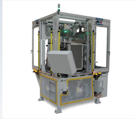
The Phoenix expands smaller-diameter copper tubes using high pressure. (Photograph Courtesy of Burr OAK Tool Inc.)
