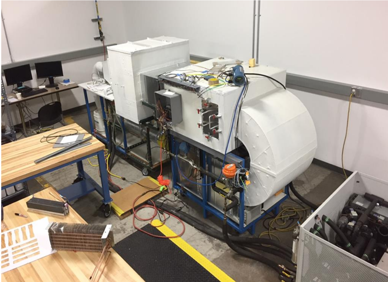
Hot water calorimeter
