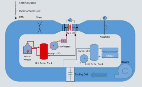
Here is a schematic of the heat exchanger test facility that was used to experimentally validate the MicroGroove correlations that are used in CoilDesigner software. Dennis Natusa from OTS presented a <u>paper on this topic</u> at the 2018 Purdue Conferences.
