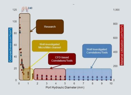
Professor Reinhard Radermacher's <u>plenary address</u> included this "Heat Exchanger Roadmap" slide, indicating the state of research on tubes of various diameters. (Image used with permission.)
