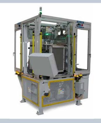
New equipment from OAK uses pressure to expand smaller-diameter copper tubes into fin plates. (Photography Courtesy of Burr OAK Tool Inc.)
